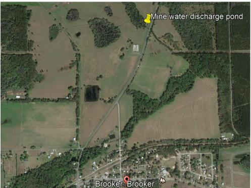
Google Earth images with mine discharge point added. Discharged water would Be through the drainage system that flows through Brooker just north of the water Tower. Flow then contines to the Santa Fe River.
