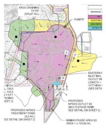
HPS II stormwater plans with proposed NPDES Outlet B3 just above substation.
